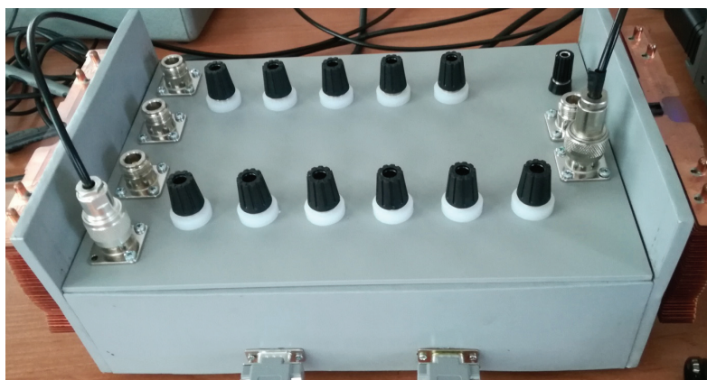
Fig. 1. New design of four-terminal single insulation transfer device
